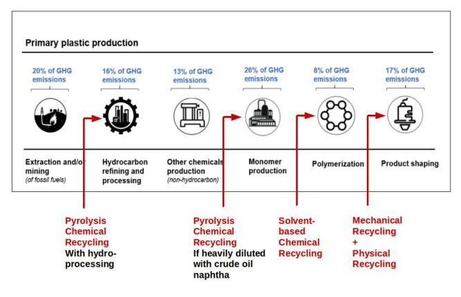
*Figure 2.* The point where the product from three different plastics recycling techniques re-enters the plastics production line. Adapted from Karali et al. (2024).
