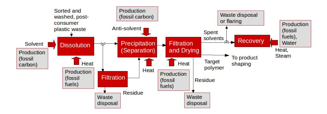
*Figure 3.* The key processing stages involved in solvent-based stripping (physical recycling) of plastics, with major environmental impacts. Note that methods vary and this is a general schematic.
