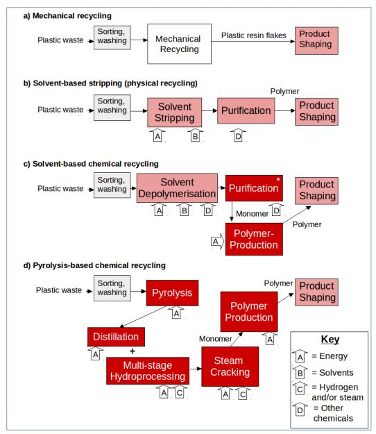
**Figure 1.** The plastic recycling hierarchy showing stages involved in each process, and significant energy and resource inputs. Darker shading indicates highest energy and resource use. Each technique is discussed in further detail, later in this report. \* = may involve multiple stages.
