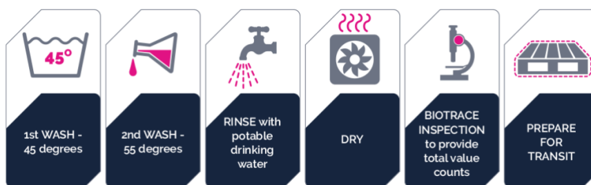
Washing process for reusable containers 15
